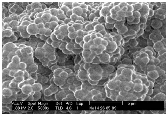
Figure 8. SEM micrographs of PMMA produced at 600 rpm.
