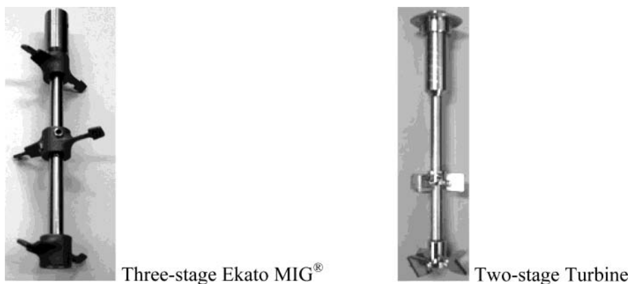
Figure 2. (a) Three-stage Ekato MIG. (b) Two-stage turbine.
